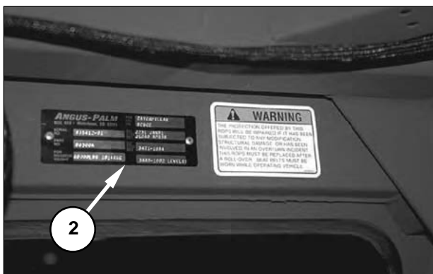
Plate (2) is located on the top right corner of the cab, inside the operator's compartment.
