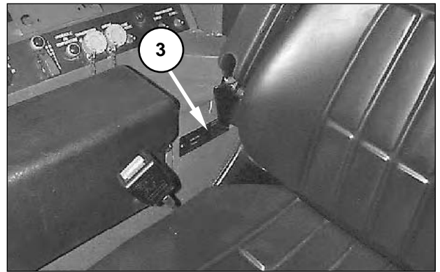
Plate (3) is located on the right control console inside the operator's compartment.
